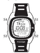
DISPLAY MODES The watch has eight display modes: TIME, COMPASS (COMP), ALTIMETER (ALTI), BAROMETER (BARO), CHRONOGRAPH (CHRO) TIMER ALARM and TEMPERATURE (TEMP).
